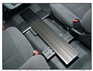
Insert 1/4" x 3/4" bolts into the bottom of Trak.
